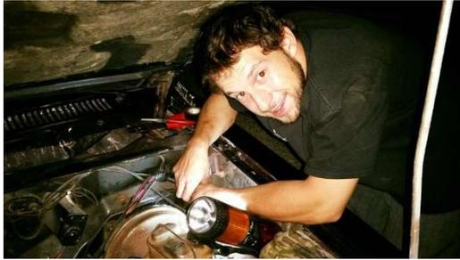
It didn't take long to conclude that we had an open circuit on the main power wire coming from the starter to the fuse block. We had to remove a few extra parts to access the wire harness and fuse block as they passed through the fire wall. One of the previous owners of the car had trouble here before and had spliced in an undersized wire to repair it. The
